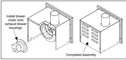
Figure 18: Exterior Exhaust Blower.
